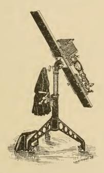
two dressed half-inch steel tubes. These tubes are placed near each edge and give rigidity as well as serve for guides for the camera and microscope carriages. In the center of the bed plate is a rack for the adjustment of the camera and microscope.
