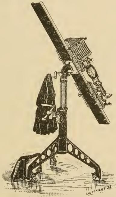
two dressed half-inch steel tubes. These tubes are placed near each edge and give rigidity as well as serve for guides for the camera and microscope carriages. In the center of the bed plate is a rack for the adjustment of the camera and microscope.
