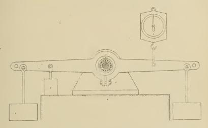
A dash-pot (H) was used to check the vibration of the lever; and the tendency of the lever to rotate, due to friction with the revolving spindle. was measured on a scale (G).
