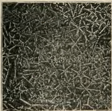
Fig. 12.—Melted at 550° C., cast in iron chilled mold. Horizontal lower section. x 50
