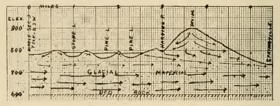
Fig. 4. Cross-section from middle of section 3, T. 36 N., R. 3 W. northward through Stone and Pine Lakes and Harding Pond, to Springville, showing probable ground water movements,
