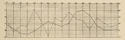
Fig. 3. Graph showing relation between the rainfall and the level of Lily Lake. Laporte, Indiana, from 1898 to 1914. Rainfall shown by broken line and referred to inches at right. Lake level shown by solid line and referred to feet at left. Datum of eity bench mark.
