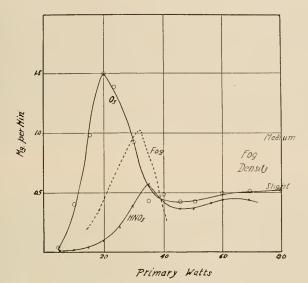
Fig. 3. The formation of ozonc, nitric acid and fog in air which was undergone discharge in contact with fragments of quartz glass; cf. Anderegg and Bowers, A Type of Silent Discharge Involving Catalysis, page 177.
