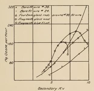
Fig. 6. Ozone formation with and without fragments of dielectric material in contact with the discharge.
