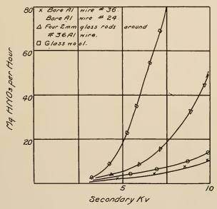
Fig. 7. Nitric acid formation with and without fragments of diclectric material in contact with the discharge.
