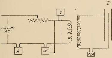
Fig. 4. Diagram of connections.
