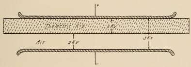
Fig. 1. The interposition of a dielectric material of constant 2 has increased the potential drop in the remaining air space from 1.5 to 2 Kv.
