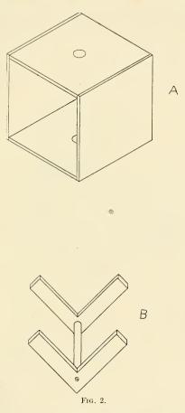
mica window the door to the ionisation chamber is constructed like that of the door to the gold leaf box. The front door should be hinged to the box and the back side can either be permanently soldered to the box or it can be fastened by means of hinges.
