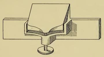
MICROTOME KNIFE.—In this drawing the two blades are shown clamped together in position for use, but without the cutting blade inserted. When the set-screw is loosened the front blade falls forward far enough to allow of the insertion of the cutting blade.
