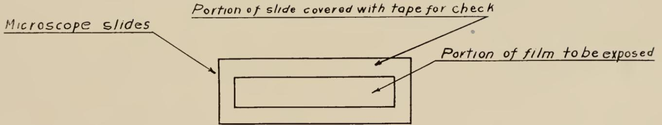
Camera plate made of two microscope slides with film of same size between Edges taped to prevent wetting and act as a check
