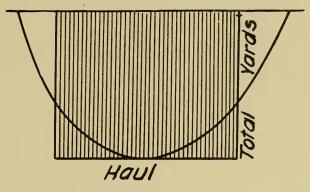
The pay haul is equal to the area of the rectangle which has for its base the haul, and its altitude the total yardage or maximum ordinate, the product of the two being also the area of the mass diagram.
