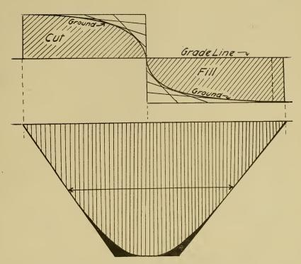
The above figure is Case III, and shows the ground a porabola in longitudinal section. This case most nearly coincides with the actual conditions, for haul, of any of the three cases, and any variance discovered here in the results of the four methods are about what would occur in actual practice, while those discovered under Case II are limiting values.
