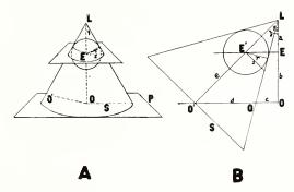
Fig. 8A and B. The projection of spherical sound waves upon a plane surface.
