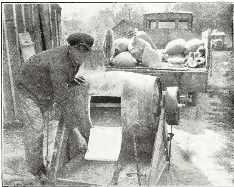
Fig. 1. One type of treating apparatus used to mix the wheat with the copper carbonate. The dust is sufficiently poisonous to cause sickness, and operators should avoid breathing it.
