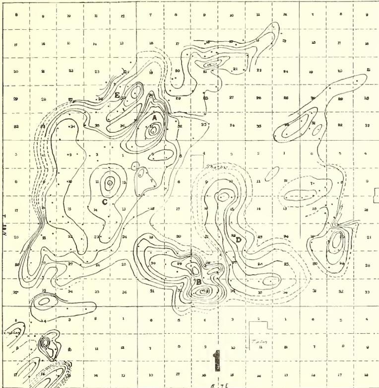
Fig. 1. Showing irregularities developed on the surface of the Cincinnati shales by using the Silurian-Ordovician contact as a key horizon. The contour interval used is 20 feet.
