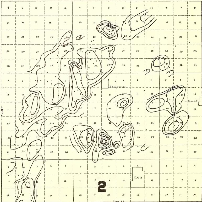
Fig. 2. Showing irregularities developed on the surface of the Mohawkian (Trenton) limestone of Ordovician Age. The key horizon used is the top of the Trenton limestone. The contour interval is 10 feet.
