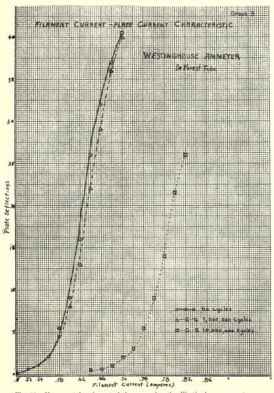
Fig. 11. Vacuum tube characteristic curve for the Westinghouse ammeter.
