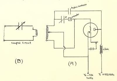
Fig. 2. The oscillator used for production of current is shown in A. The heat apparatus and ammeters to be calibrated were connected in the tuned circuit shown in B.
