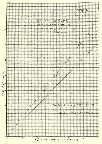
Fig. 4. Calibration curve for the Westinghouse ammeter (type px-2).
