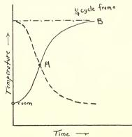
Fig. 7. Modification of curves if a simple harmonic alternating current is used instead of an intermittent direct current.
