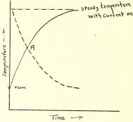
Fig. 6. Cooling follows a symmetrical curve (dotted) when current is stopped after the temperature has reached the point P.
