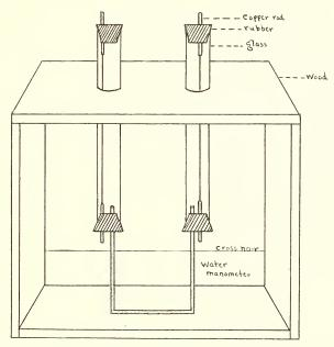
Fig. 1. Device used in the investigation for the calibration of ammeters.
