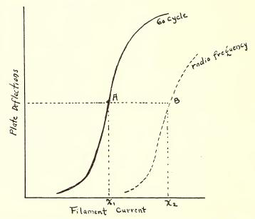
Fig. 10. By comparing the two characteristic curves obtained, the true value of the radio frequency current through the filament is determined.
