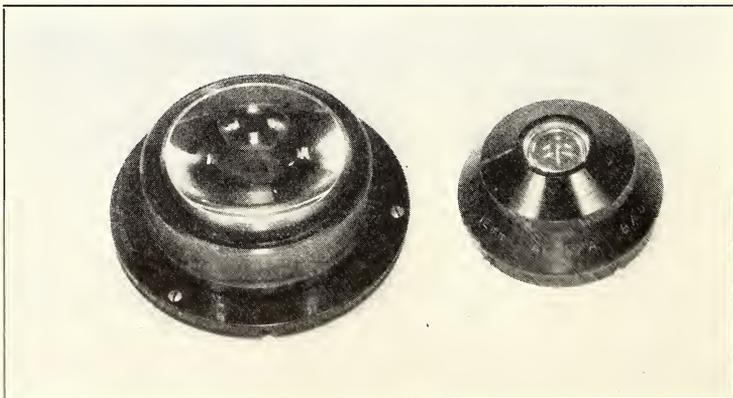
Fig. 2. Aplanatic substage condenser removed and separated. The larger unit is for low power work; as a doublet it is used for high power work.
