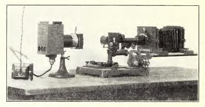
Fig. 1. Photomicrographic equipment assembled.
