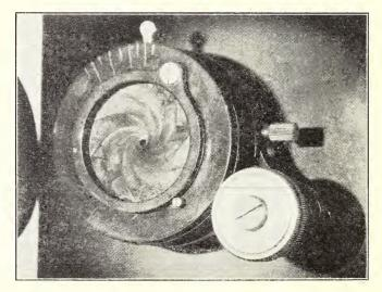
Fig. 4. The substage diaphragm closed. Stops are marked on the plate.
