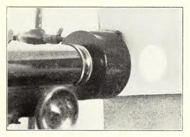
Fig. 3. Focusing the light through the ocular on a piece of paper held back of the ocular.
