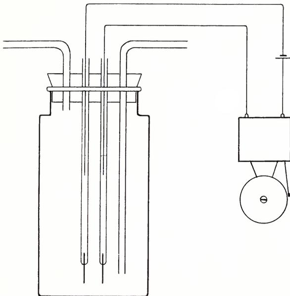
any evolved gaseous ammonia into running water. This arrangement is satisfactory in most instances. At times, however, water is sucked back into the ammonia. An ordinary trap bottle is of little value here, for when placed in the gas line it merely catches water until full, and then ceases to operate. For this reason the bottle must be constantly watched in order to detect any flow of water into the system.
