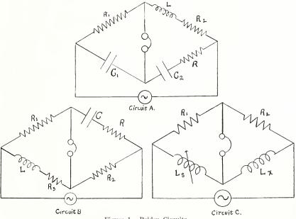
Figure 1. Bridge Circuits.
