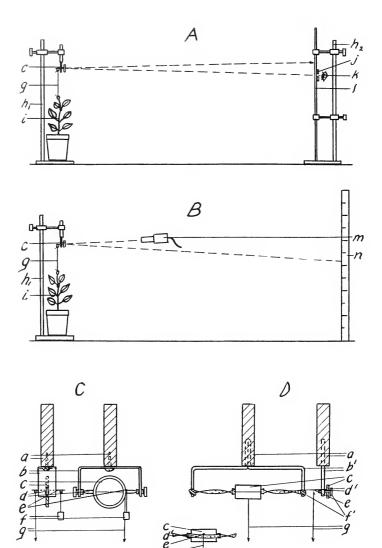
Fig. 1. Optical lever apparatus. (a) wooden handle, (b) metal frame, (b) heavy wire frame, (c) mirror, (d) mirror axis, (d) rubber band, (e) lever arm, (f) counter balance weight, (f) adjusting peg, (g) connecting cord leading to plant, (h<sub>1</sub>) and (h<sub>2</sub>) ring stands, (i) plant, (j) card board light stop with sighting aperture, (k) eye, (l) meter stick, (m) light source, and (n) large scale.
