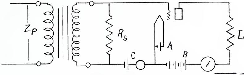
Fig. 4. Transformer circuit for primary impedance.
