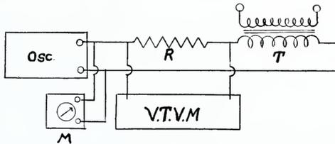
Fig. 8. Current determining circuit for series resonance.
