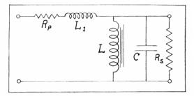
Fig. 2. Equivalent circuit of audio transformer.
