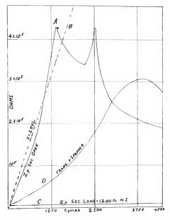
Fig. 1. Impedance curves for output transformer.
