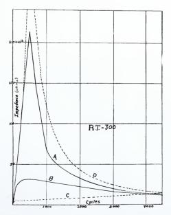
Fig. 6. Impedance curves for interstage transformer.
