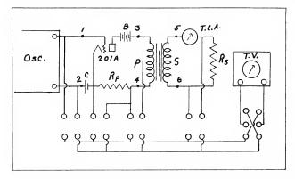
Fig. 3. Measuring circuit for transformer characteristics.
