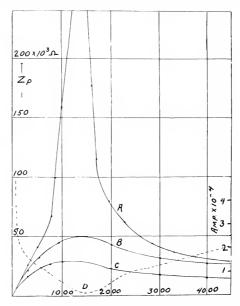
Fig. 7. Series resonance curves.
