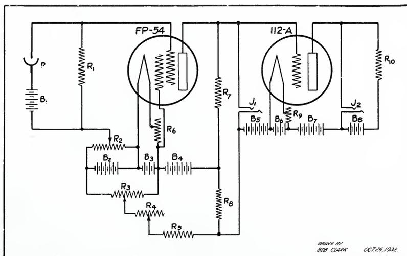
Fig. 1. Circuit Diagram. P, Photocell;  $R_1$ ,  $4.23 \times 10^9$  ohms;  $R_2$  and  $R_3$ , 400 ohm potentiometers;  $R_4$ , 2500 ohm;  $R_5$ , 20,000 ohm fixed resistance;  $R_7$  and  $R_8$ , 10,000 ohm fixed resistances;  $R_6$ , 50 ohm;  $R_9$ , 6 ohm;  $R_{10}$ , 2500 ohm variable.  $B_1$ , 90 volts;  $B_2$ ,  $B_3$ ,  $B_6$ , 6 volt storage batteries;  $B_4$ , 2 volt storage cell;  $B_5$ , 9 volts;  $B_7$ , 135 volts;  $B_8$ , 4.5 volts.
