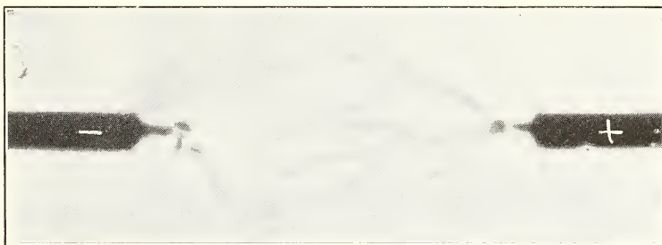
Fig. 4—Discharge terminates in glow at positive terminal.
