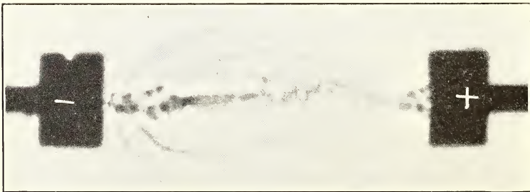
Fig. 3—Vapor being projected in form of globules and molecular aggregations.
