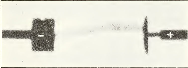
Fig. 6—Striations in an ancient spark due to a weak discharge.
