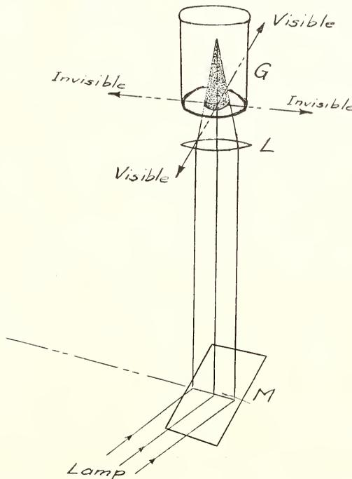
Fig. 1.—Diagram of apparatus used to demonstrate the theory of scattering of polarized light by small particles.
