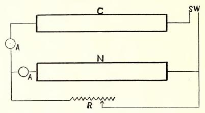
Fig. 2-Diagram of apparatus used in insulation tests.
