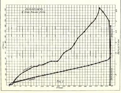
Fig. 1-Stress-Strain and Stress-Deflection curves for mild steel.
