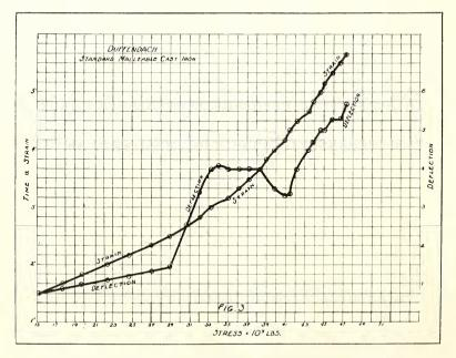
Fig. 3-Stress-Strain and Stress-Deflection curves for malleable cast iorn.
