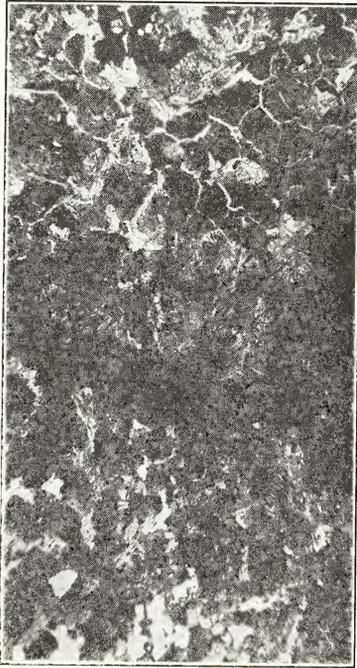
Fig. 1—Structure of the case formed on ingot iron by heating to 950° C. for 5 hours in a commercial carburizing material.
