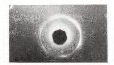
Fig. 2. X-ray diffraction of paraffin film on end of glass tube. Orientation pattern indicates formation of large crystallites and orientation of a long chain normal to the plane of the film.
