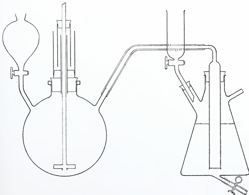
Fig. 1. Apparatus for the Synthesis of Ethyl Acetylene.
