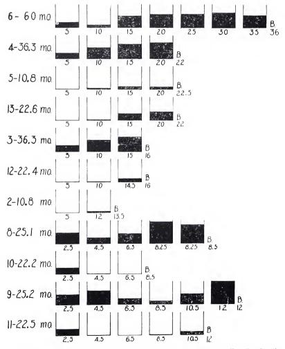
FIG. 5. Graphic representation of total weights of sediment collected. On the extreme left are the collector numbers, followed by the number of months the collector was in the lake. Under each jar is its depth in meters below the surface; under B, at the end of each series, is indicated in meters the depth of the lake at that point.
