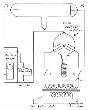
Fig. 1. Complete set-up for both half and full wave rectification.
