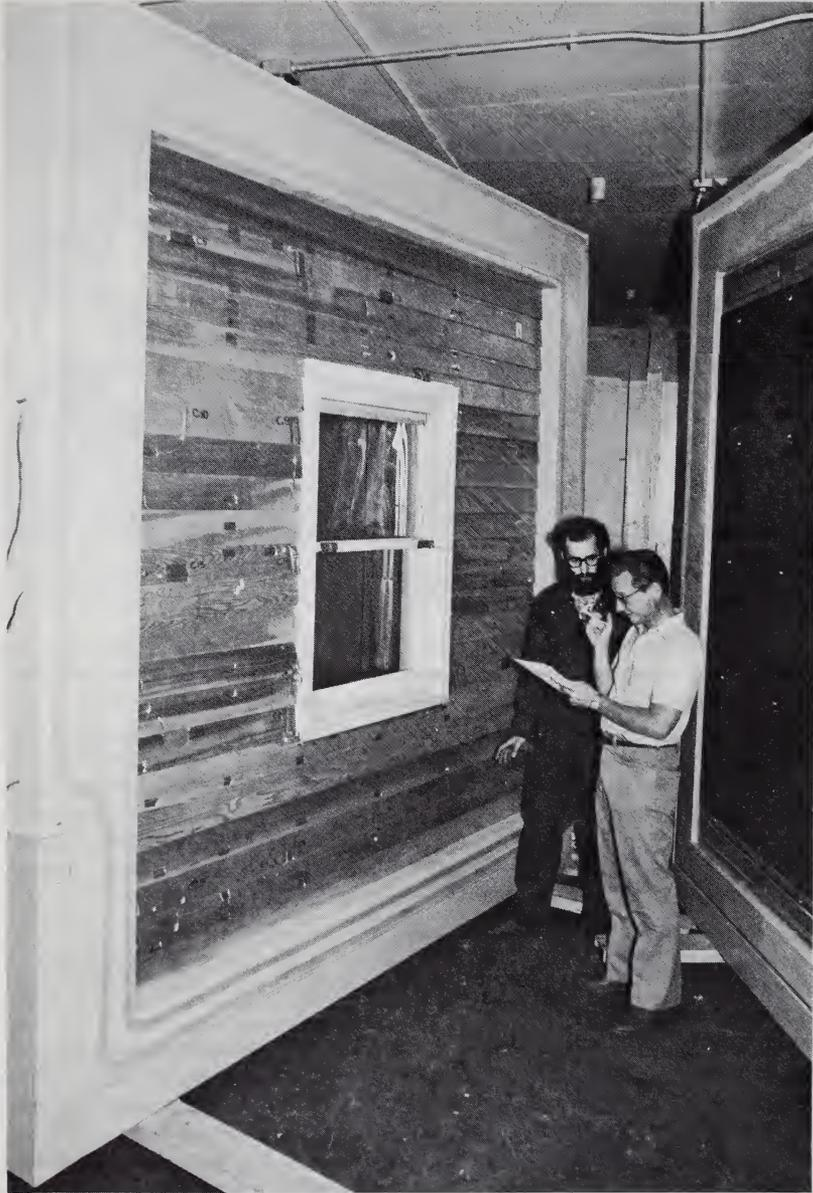
FIGURE 8. *Thermal Resistance Measurement System*
