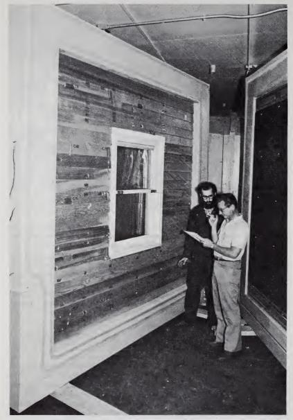
FIGURE 8. Thermal Resistance Measurement System
