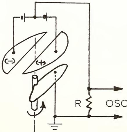
Figure 2. Split plate capacitor.
