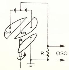
Figure 2. Split plate capacitor.
