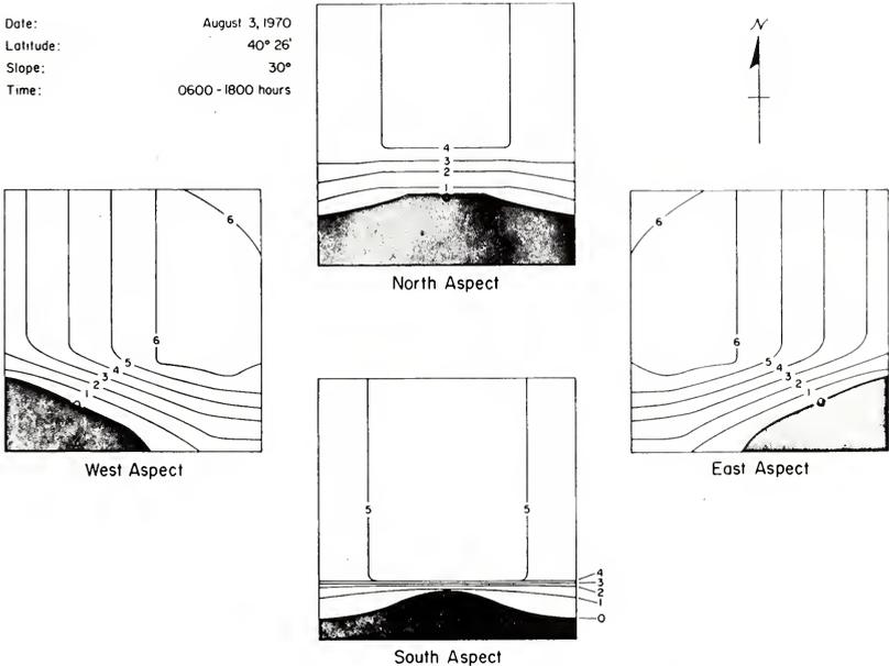
FIGURE 3. The effect of aspect on sunlight duration patterns in  $1\frac{1}{2} H$  square openings. Other problem variables are given in the figure. The contour interval is one hour. The darkened areas represent those portions of the opening not receiving direct sunlight during the 12 hour time period.
