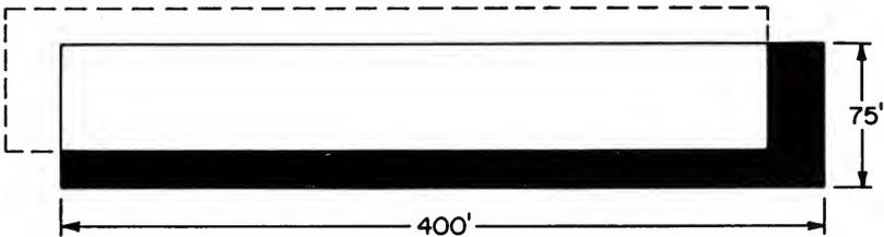
FIGURE 1. A simulated forest opening shadow pattern. The solid line indicates the opening map. The darkened area is in shade at the simulated time. The dashed line borders an area on the forest floor outside the opening that is potentially in the sun.
