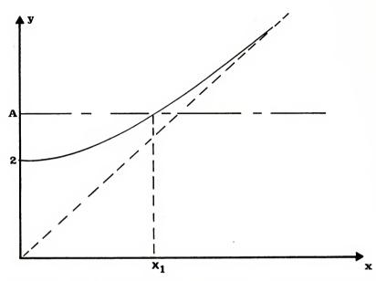
FIGURE 2. Sketch of the graph of  $y=xIo(x)/I_1(x)$  for x > 0, from which it is clear that the equation y = A has one and only one real solution  $x_1$  (say) for every constant A > 2.
