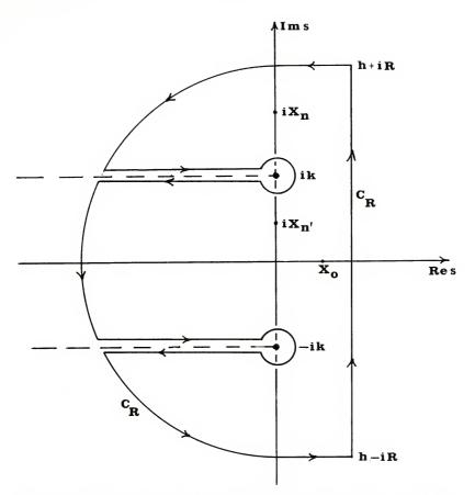
FIGURE 5. The contour CR for inversion of the transform Ez (r,s,w) in § 4. The contour avoids the purely imaginary branch points ±ik, as well as the simple poles iXn lying on the Im s axis. (iXn denotes those poles < k in absolute value.) In the limit as R→oo and the radii of the small circles about ±ik tend to zero, the right-hand side of [23] tends to the wanted field components Ez (r,z,w).</p>
