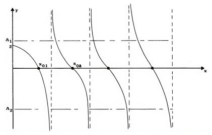
FIGURE 3. Sketch of the graph of  $y=xJ_{\theta}(x)/J_{1}(x)$  for x>0. The points  $x_{\theta}k$  are the zeros of  $J_{\theta}(x)$ . (The vertical asymptotes occur at the zeros  $x_{th}k$  of  $J_{1}(x)$ .) It is clear from the sketch that the equation y = A always has countably many real solutions for every real A. If  $A = A_{2}<2$ , then there is a real solution on the interval  $0 < x < x_{11}$ . If  $A = A_{1}>2$ , then there is no real solution on this interval.
