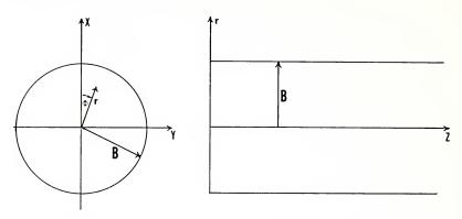
FIGURE 1. From left to right, cross- and longitudinal sections of the domain V:  $O \leq r < B_r/z < \infty$ . The wall impedance boundary conditions are applied at r=B.
