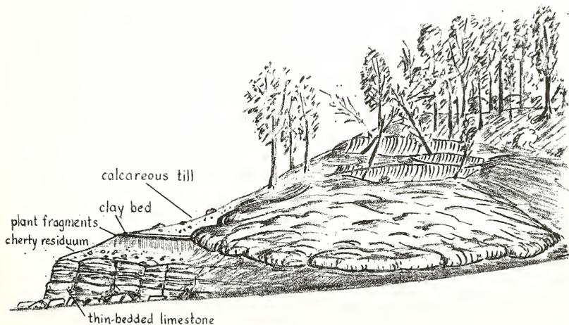
Figure 2. Terrain sketch and diagram of the geology along State Road 46 in Owen County where mudflows and slump have resulted from an over-steepened slope and a perched water table held by a thin Pleistocene clay bed.
