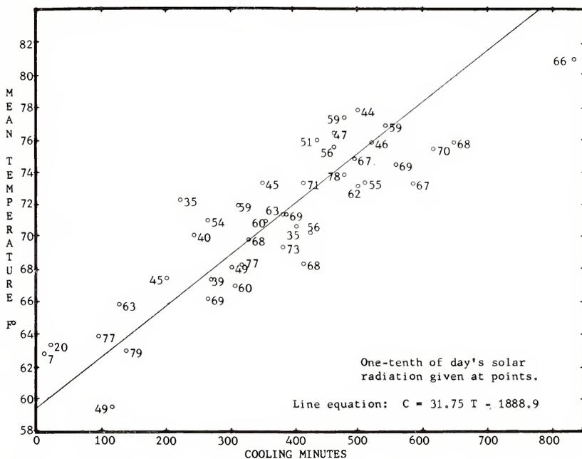
FIGURE 1. Daily observations of outdoor mean temperature are related to minutes of cooling to maintain a temperature of 78°F or lower in a typical dwelling. The day's solar radiation in tens of calories per square centimeter is given at the point. Cooling minutes accumulated when the daily mean temperature exceeded 59°F generally.
