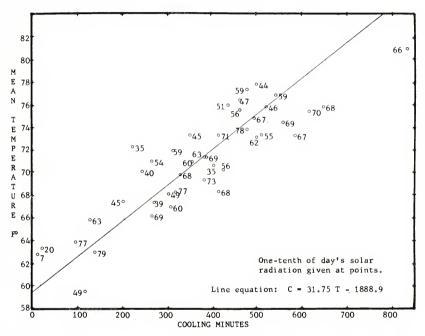
FIGURE 1. Daily observations of outdoor mean temperature are related to minutes of eooling to maintain a temperature of  $78\,^{\circ}\text{F}$  or lower in a typical dwelling. The day's solar radiation in tens of ealories per square centimeter is given at the point. Cooling minutes accumulated when the daily mean temperature exceeded  $59\,^{\circ}\text{F}$  generally.
