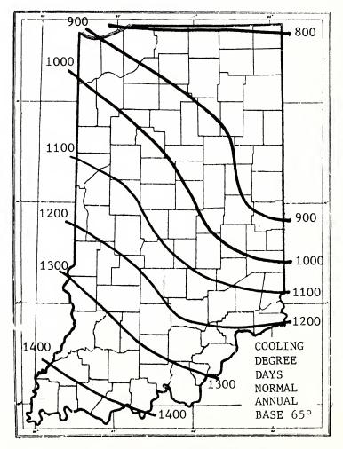
FIGURE 2. Normal annual cooling degree days calculated from daily mean temperatures above  $65^{\circ}F$ .
