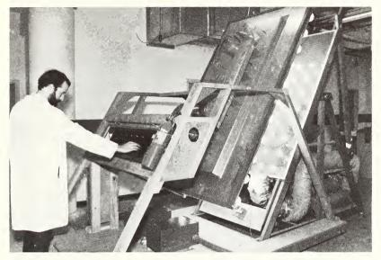
FIGURE 7. Solar Hot Water Collector under Test at the Indianapolis Center for Advanced Research
