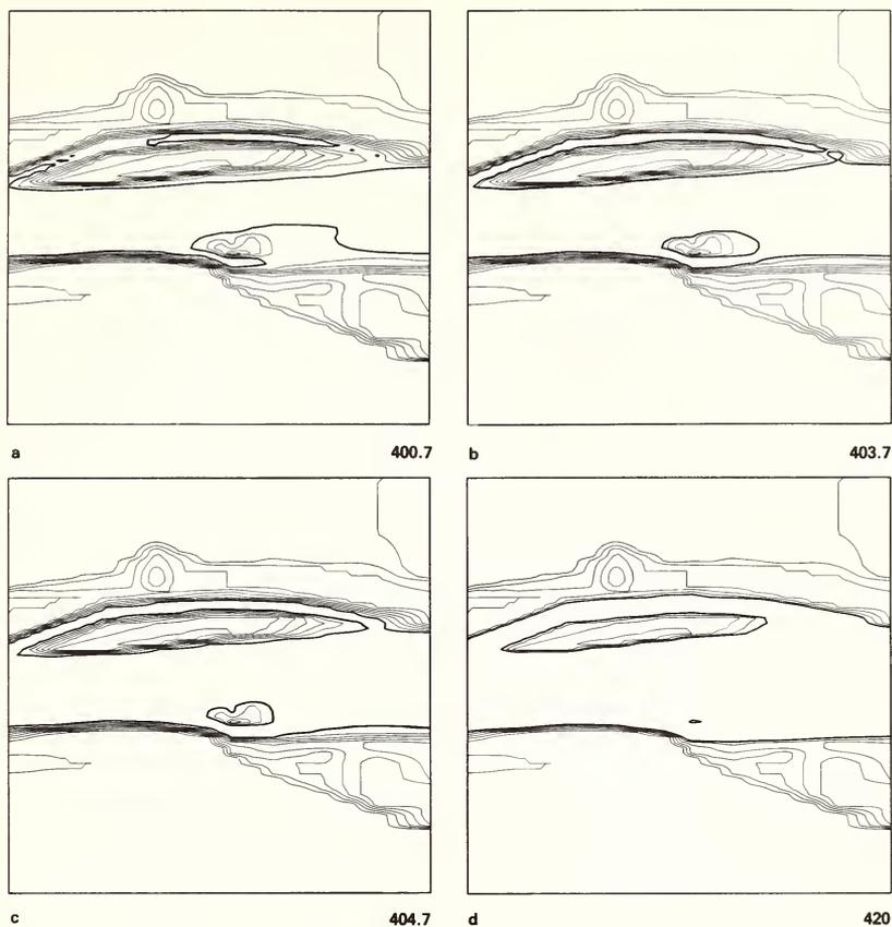
FIGURE 1. *Shoreline configuration near Sixmile Island: a. at stage 400.7 ft, when the Louisville Chutes were dry; b. at stage 403.7 ft, this paper's upper estimate for the 1792 low water mark; c. at stage 404.7 ft, low water mark of 1895 when a wing dam was present; d. at stage 420, ft, nowadays normal pool level, after the construction of McAlpine Dam.*
