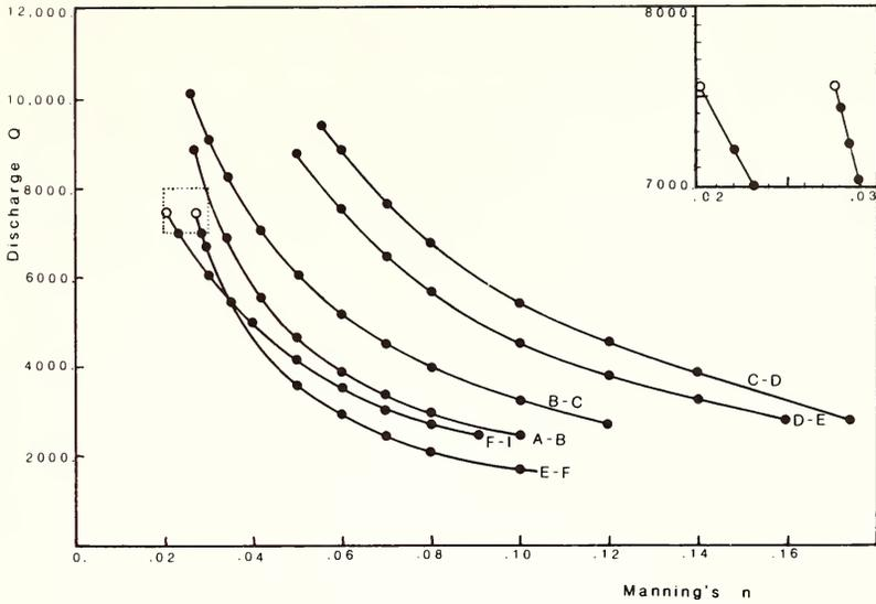
FIGURE 6. The Ohio Chutes trunk's loci of the couples  $(Q,n)$  which yield the measured stages at both ends of each trunk.
