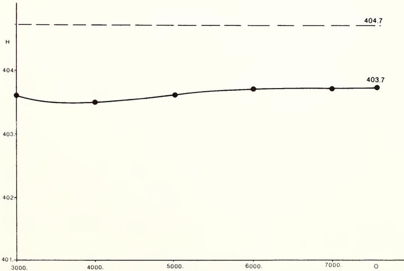
FIGURE 7. Pool elevations corresponding to different discharges (and different roughnesses).
