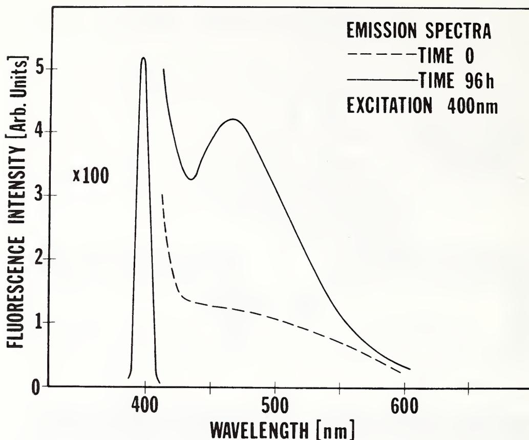
FIGURE 3 Representative fluorescence emission spectra of irradiated tissue as measured by the *in situ* light guide probe shown in Figure 1 and Figure 2.
