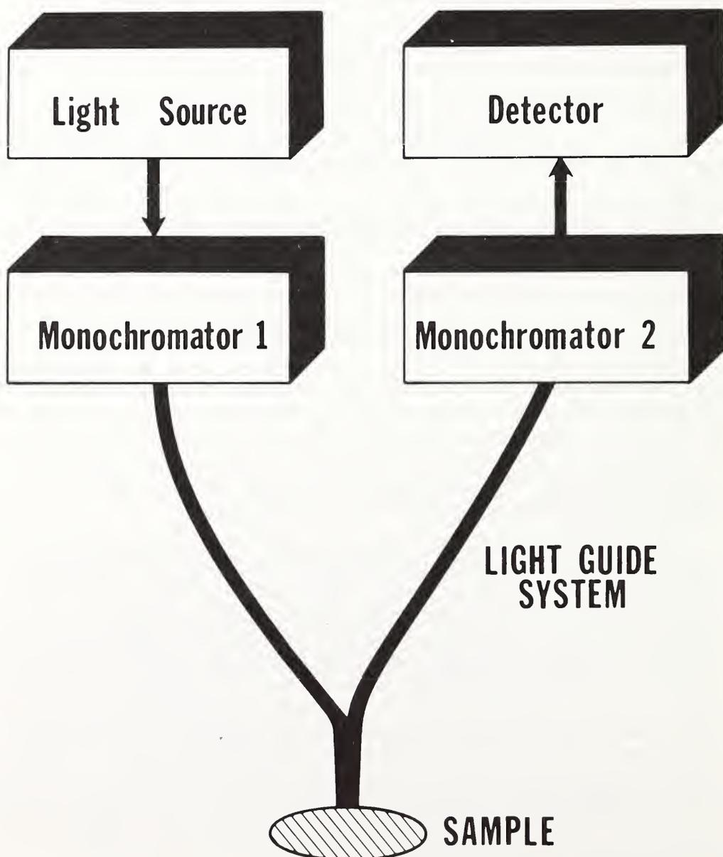
FIGURE 1 *Block diagram of in situ fluorometer.*
