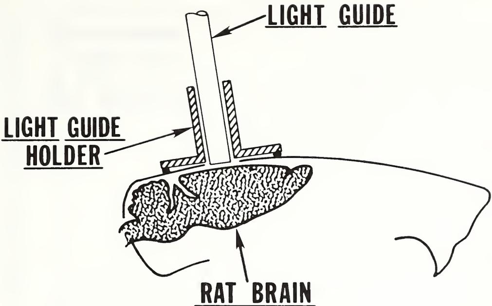
FIGURE 2 Cross section diagram of a rat skull showing approximate positioning of the light guide.
