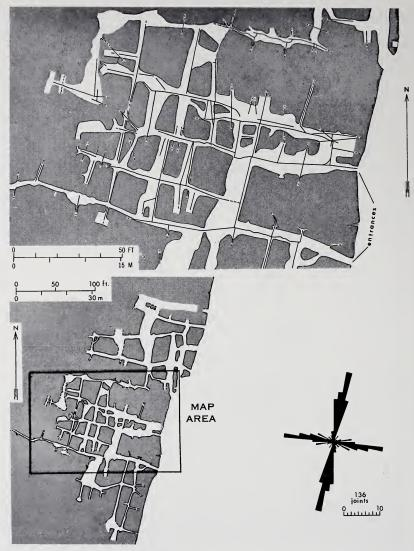
FIGURE 4. Map of a portion of Herron Cave, Crawford County, in the Glen Dean Limestone, showing the pattern of master and cross joints in relation to cavern passages. The rose histogram was compiled from 136 joint measurements and represents the entire cavern.
