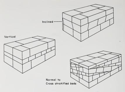
FIGURE 1. Block diagram showing three basic types of jointing.
