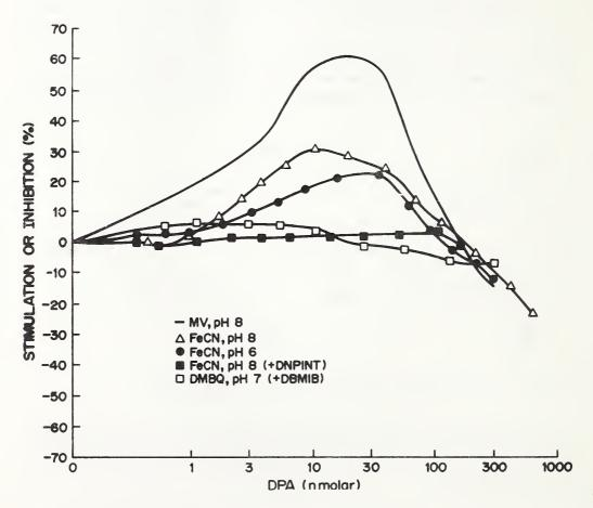
FIGURE 2. Uncoupling of Photosystem I and II Reactions by the Uncoupler, DPA. Reaction mixtures contained chloroplasts (0.05 mg chlorophyll), 25 mM Tris-Mes, pH 6, 7, or 8, as shown and electron acceptors or inhibitors in concentrations indicated below: DMBQ-10mM; DCMU-5 $\mu$ M; DNP-INT; 10 $\mu$ M; and FeCN 250 or 500  $\mu$ M.
