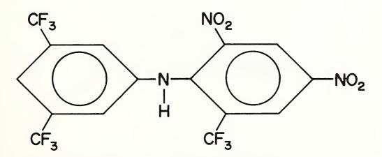
FIGURE 1. The Chemical Composition of the Uncoupler, DPA.
