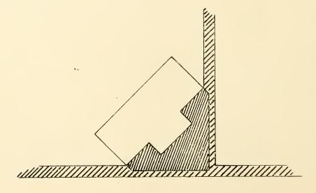
SEC. 45. Ends of joists or beams entering a brick wall shall be cut so as not to disturb the brick-work by any deflection or breaking of the joists or beams. All such joists or timbers entering a party or division wall from opposite sides, shall have at least four (4) inches of solid brick-work between the ends of such timbers
