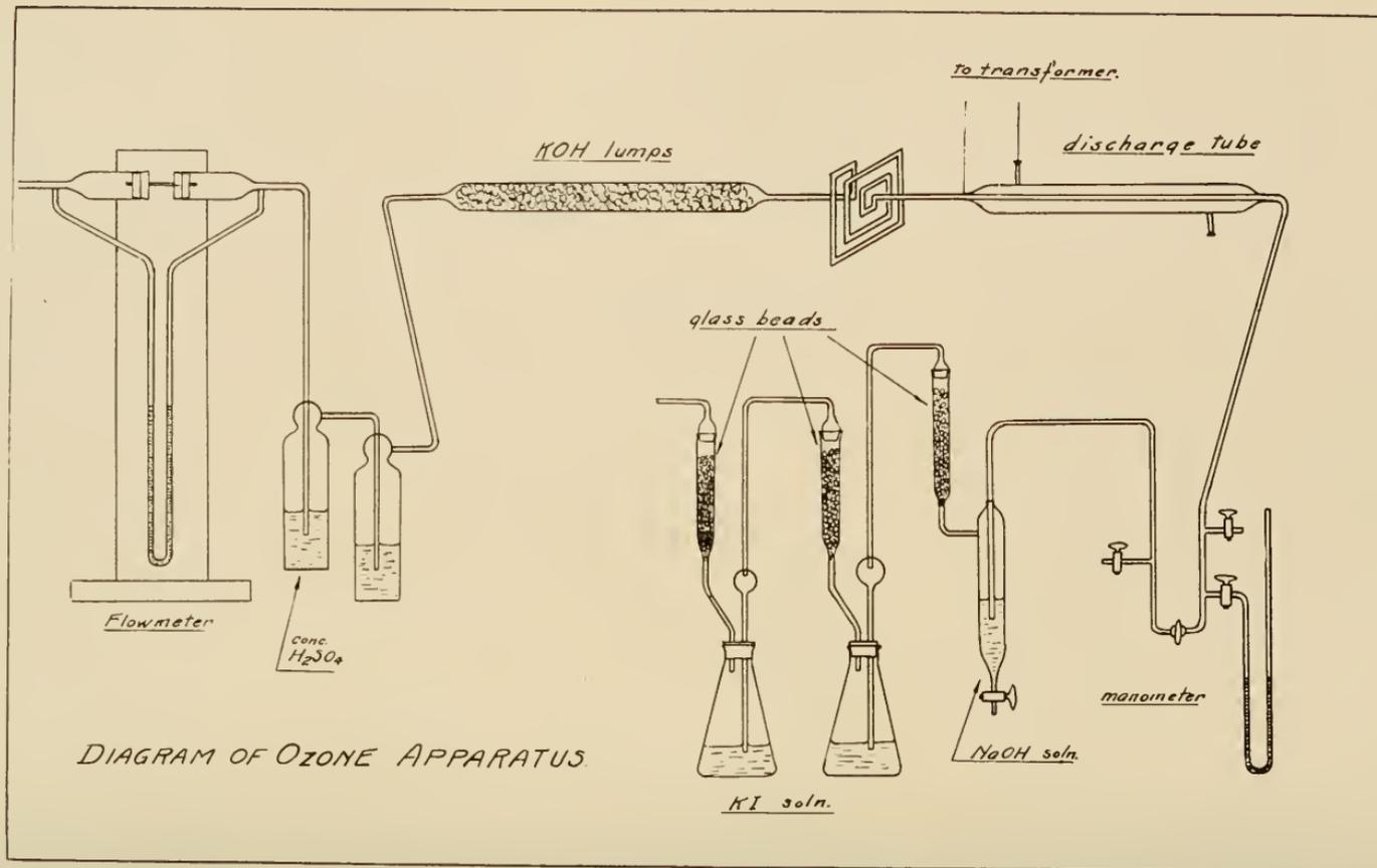
Fig. 5. Diagram of ozone apparatus.
