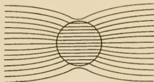
Fig. 2. The lines of force in an electric field are distorted by a rod or sphere of dielectric material.
