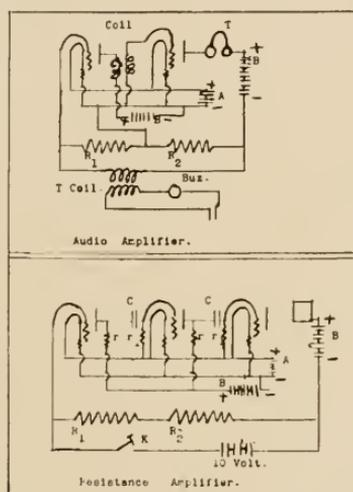
Fig. 1. Diagram of audio and resistance amplifiers.
