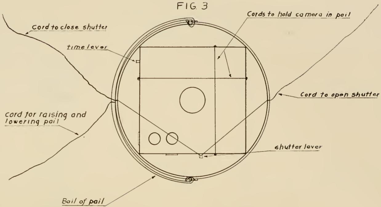
Top view of under water camera apparatus showing camera in position and means of operating.
