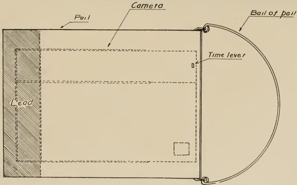
Side view of under water camera apparatus showing camera in position and means of operating.
